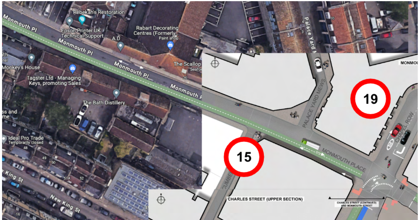
16. Monmouth Place/Charlotte St: Tighten junction significantly creating a safer junction for crossing by pedestrians and better junction interaction for cyclists.
